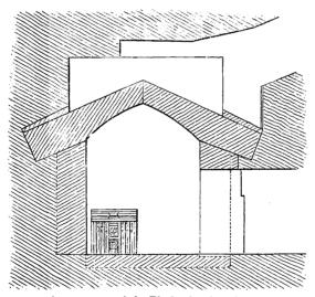
Arrangement of the Blocks forming the Roof.
