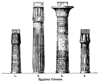
The column bulges out from its base like a water-plant, and is then sculptured so as to resemble a number of stalks tied together at the top or at intervals, and finally swelling above the last compression into a calix.<sup>3</sup> Or it has the leaves and flowers of water-plants delicately traced upon it and coloured naturally.<sup>4</sup> Or, finally, it retains the mere general form derived from pillars thus moulded, and substitutes
