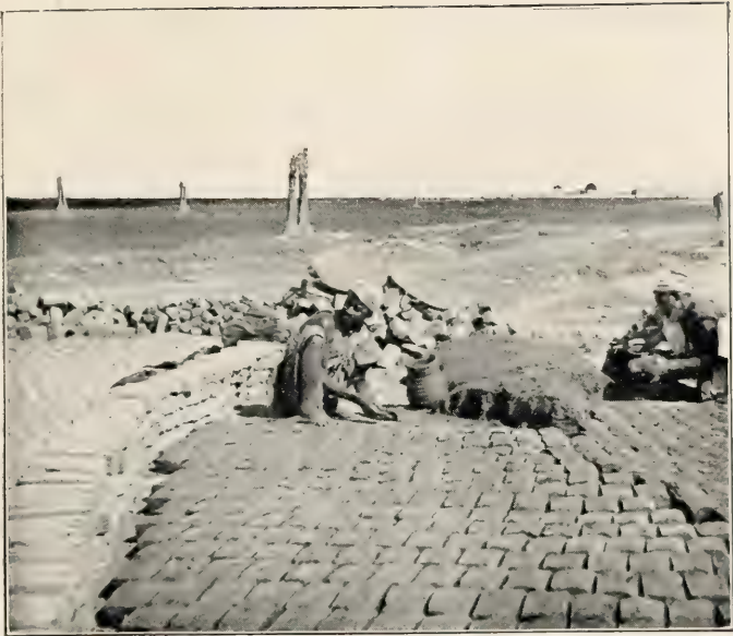
FIG. 11.—Modern Egyptians making bricks. Note the mat beyond the man for carrying the mud, the mound of mud, the water-pot for wetting the mould, the rows of bricks drying on the ground, and the dry bricks stacked on the right.
