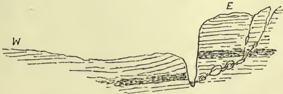
FIG. 2.—Diagram of great fault, eroded into a gorge, fed by water-tunnelled caverns in the cliffs.
