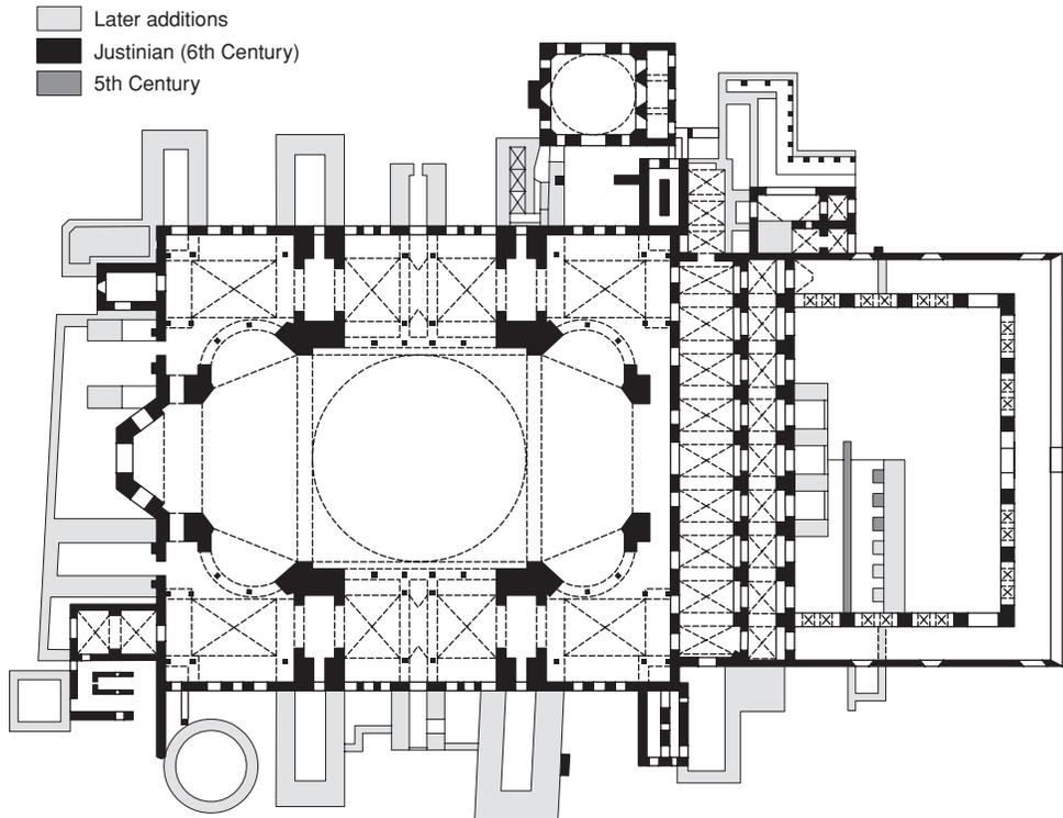
**Figure 6.2** Hagia Sophia, plan. The plan of Hagia Sophia tells us a great deal about the building. The core of the building was conceived at floor level as a large rectangle, 78 x 72 meters, with side aisles along the north and south, separated from the central aisle by an enormous colonnade. Thus, in some sense it was a basilica. Four massive piers supported a central dome, 100 Byzantine feet (31 meters) in diameter, and two half-domes on the east and the west
